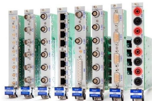
Figure 5: Acquisition and Amplifier Modules [8]
